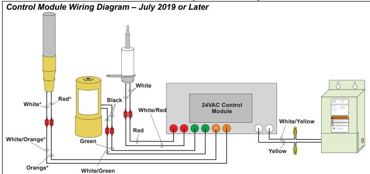
\* NOTE: The thermopile must connect to the control module as shown above (white/orange wire connects to the white thermopile wire and orange wire connects to the red thermopile wire). Do not reverse the wires. If the wires are reversed, the torch will not work correctly.
