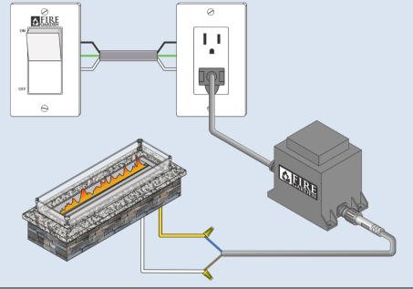
• The transformer is plugged into a GFCI-protected, non-switched outlet. One low-voltage conductor is interrupted by a switch. The low-voltage conductors are then attached to the yellow and white wires from the control module. Polarity does not matter for any of these connections.
