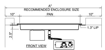
SPARK IGNITION BY AA BATTERY MATERIAL: 304 STAINLESS STEEL
